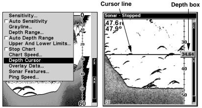
Sonar Page menu with Depth Cursor selected (left). Chart with depth cursor active (right). Cursor line shows the large fish is 34.64 feet deep. The cursor can be moved to any location on the screen, letting you pinpoint the depth of a target.
